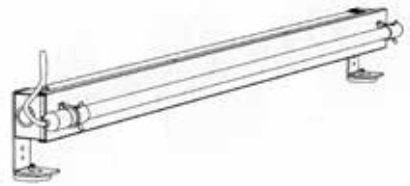
Fig. 6 Magnet mount installation with magnets on the short side of the bracket
