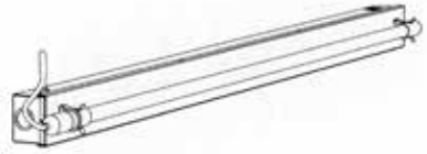
Fig. 5 Direct mount installation allows unit to be bolted directly, without need for brackets.
