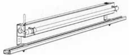
Fig. 4 Strut mount installation with unit bolted to the strut on the short side of the bracket.
